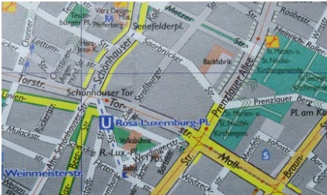
Berlin cycling map showing cycle streets (green-yellow), cycle facilities (yellow), cycling on bus lane (orange), calm streets (white), uncomfortable surface / very busy road (grey) © Tilo Schütze, www.baerleinplan.de
